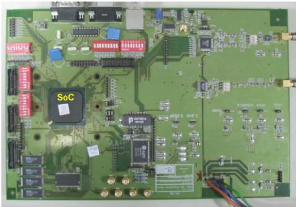
Fig. 7. Reference board hosting the implemented SoC
